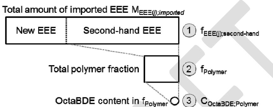
**Figure 4-3:** Scheme to estimate the amount of c-OctaBDE in imported EEE
