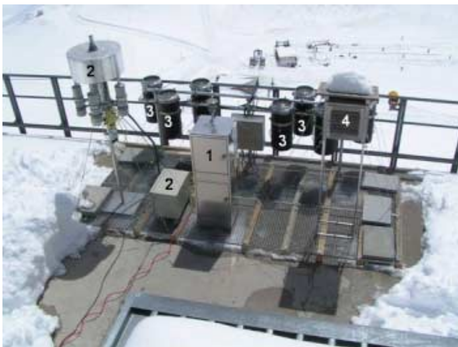
1...low volume sampler, 2...high volume sampler, 3...deposition samplers, 4...SPMD passive sampler
